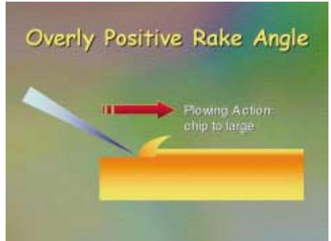
FIGURE 6 Overly positive rake angles.
